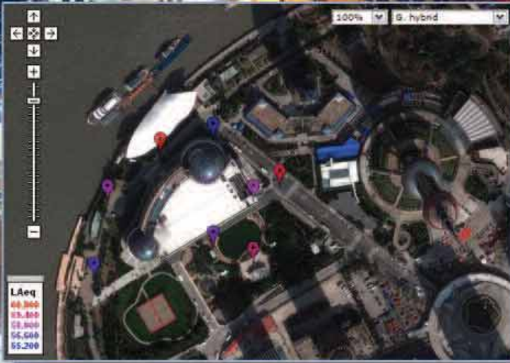
Fig. 10 Noise map created using web-based GPS mapping
