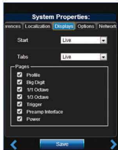
Fig. 8 Customizing Model 831 Instrument Displays utilizing SLM Utility-G4 Software
