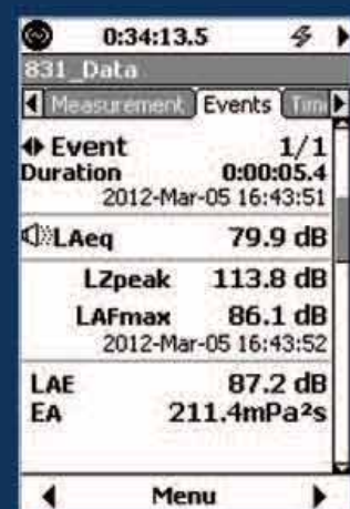
Fig. 22 Event Detection Display on the Model 831
